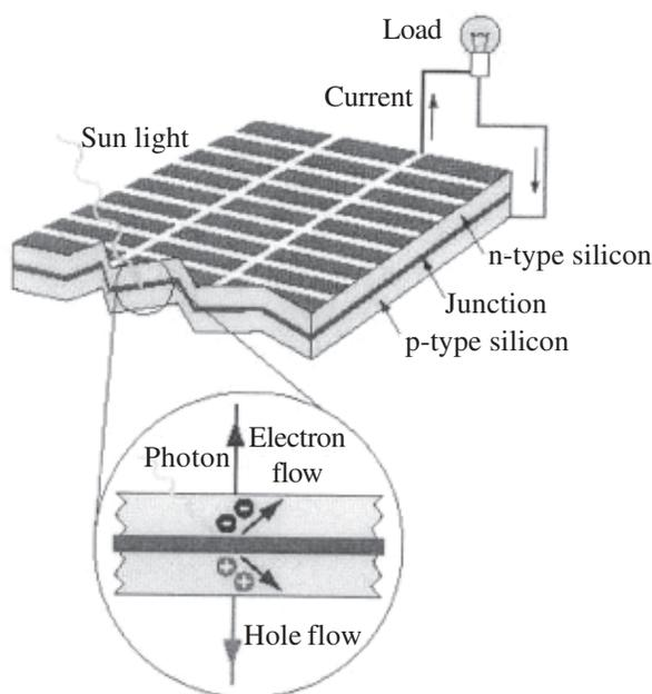
*Fig. 29.3: Photovoltaic cell*
