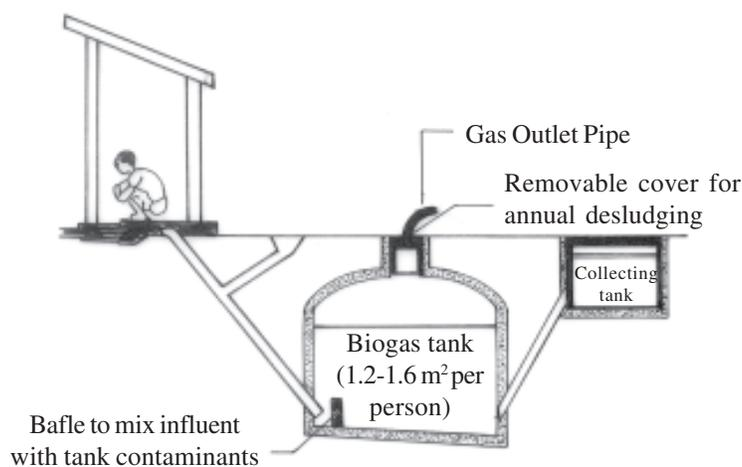
**Fig. 30.2:** Biogas Plant
