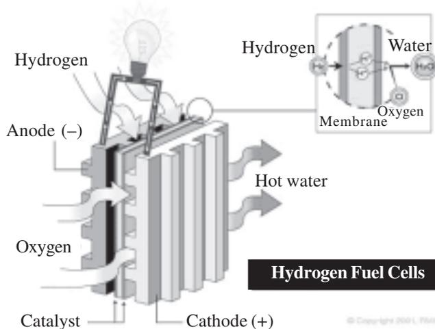
**Fig. 30.8:** Structure and function of fuel cell
